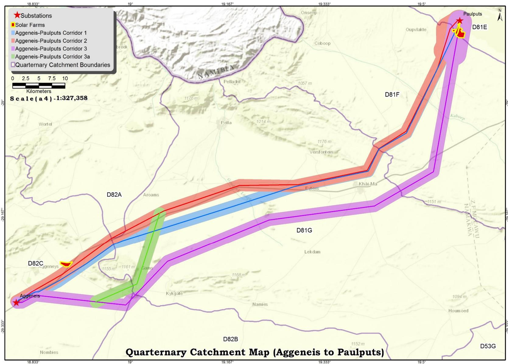
Figure 2 Route corridor alternatives associated with the 400kV Aggeneis-Paulputs power line and their quaternary catchments.
